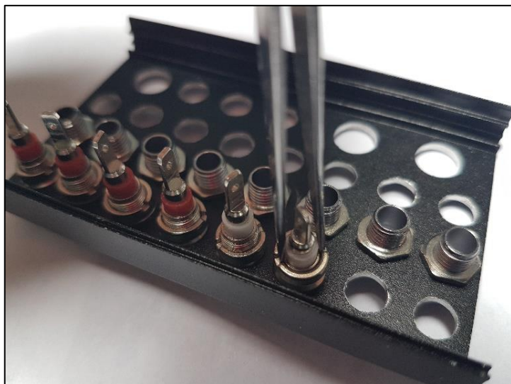
Figure 22 – Tightening the connector nuts
